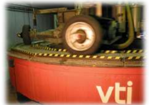
Figure 5.1: The VTI circular road simulator Pavements in the road simulator: Czech diorite (top) and Slovenian limestone (bottom)
