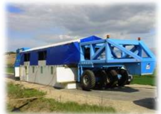
Figure 2.1 Heavy Vehicle Simulator
