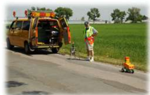
Figure 2.2 Bearing capacity measuring devices
