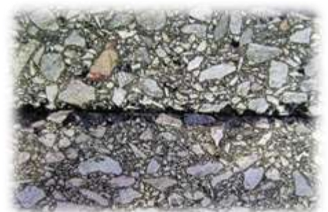
Figure 5.2: Pavements in the road simulator: Czech diorite (top) and Slovenian limestone (bottom)
